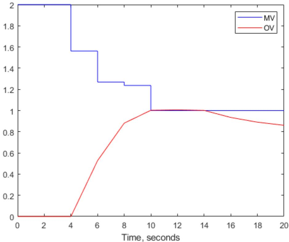
From the plot, you can observe that the original MV upper bound is active until  $t = 4$ . After the input delay of 4 seconds, the output variable (OV) moves smoothly to its new target of  $r = 1$ , reaching the target at  $t = 10$ . The new MV bound imposed at  $t = 10$
