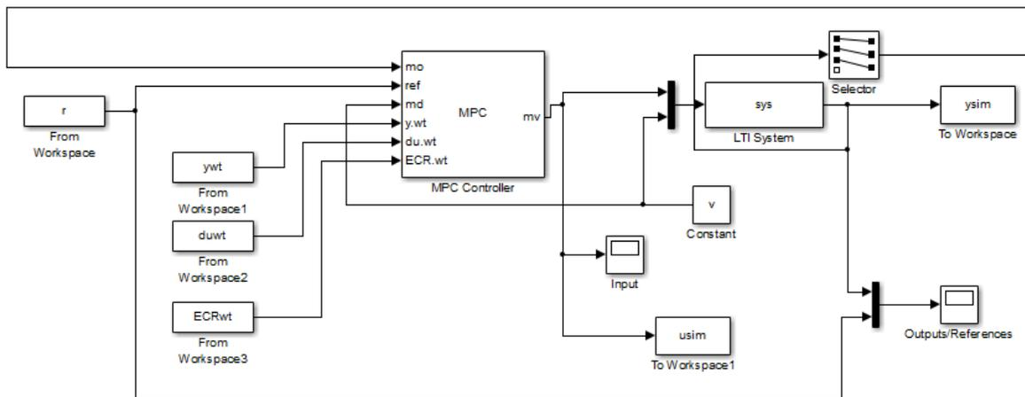
Add an inport (`y.wt`) that you can connect to a run-time output variable (OV) weight signal. This signal overrides the `Weights.OV` property of the `mpc` object, which establishes the relative importance of OV reference tracking.
