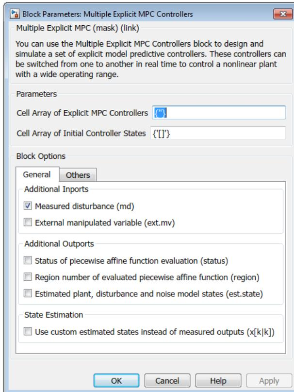
The Multiple Explicit MPC Controller block has the following parameter groupings:
