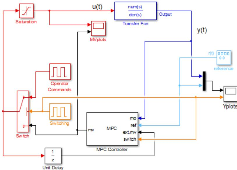
If the external MV option is inactive or the `ext.mv` input is unconnected, the controller assumes that its MV output is used in the plant without modification.
